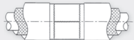
Inserting and gas-tight welding of the adapter piece
